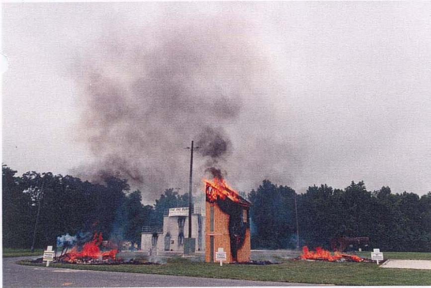
**Structure with cellulose insulation resisted the fire 57% longer than the fiberglass structure.**
