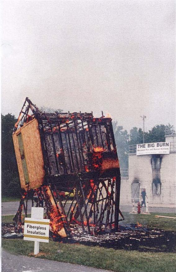
Structure with fiberglass insulation collapsed 42:26 after ignition.
