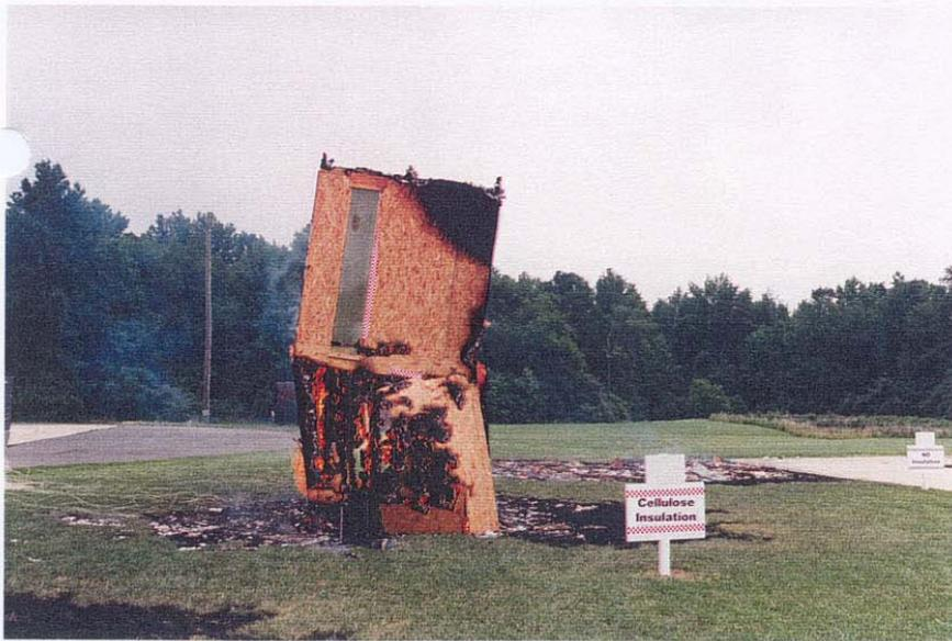
Structure with cellulose insulation collapsed 66:45 after ignition.
