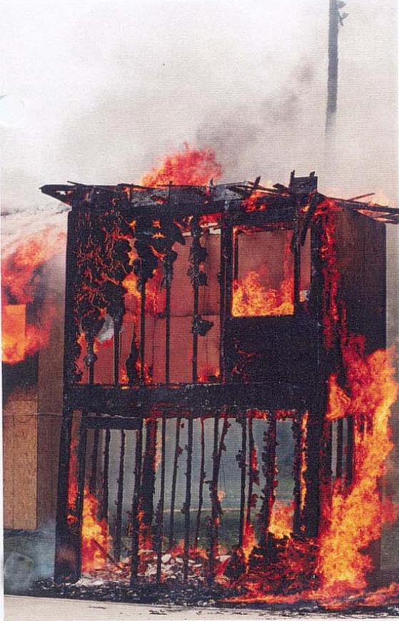
**Structure with no insulation collapsed 40:10 after ignition.**
